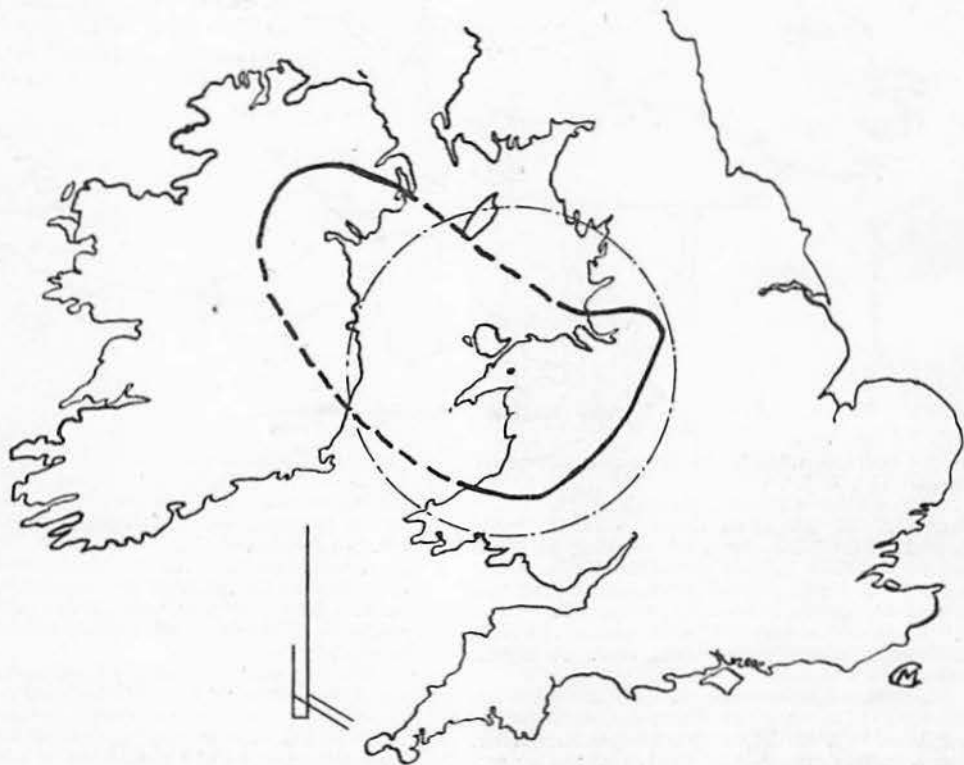
Polar Diagram. Half-wave Vertical.
